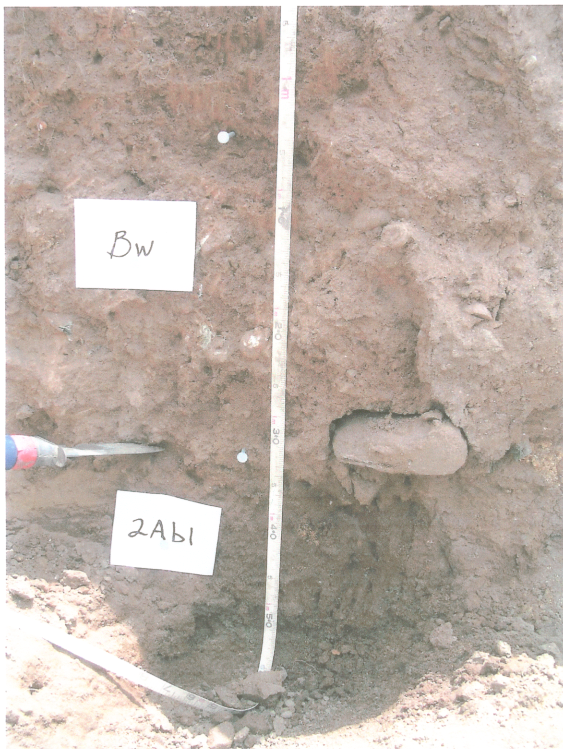
Photo 4. Relatively sharp contact between the modern soil and paleosol b1 in Soil Profile No. 4. Rocks above the contact at 132 cm appear to be part of the debris phase that followed the most recent earthquake (event W) when it produced a >132 cm vertical offset along the fault. Note flat-lying orientation of 10-cm long cobble to the right of the scale. View east. Scale in cm.
